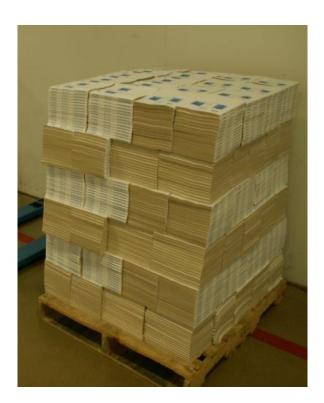
Exhibit 2. The NDC would like to receive 20 pallets of P-17 palletized according to the picture to the left. Cardboard would need to be placed on pallet before stacking to ensure stable foundation.
